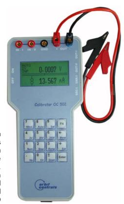
OC502 can be software calibrated via the keyboard whenever required. The instrument is supplied from internal rechargeable battery which permits 4 hour uninterrupted operation. A sign BAT at the display reminds the operator to charge the battery as soon as the voltage is bellow the secure operation value.
